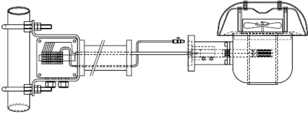
5.3 Join the connectors of the probe and mounting arm. The small two-pin connector serves for the fan supply. For probes without plugs: Loop the cable into the connection box and wire according to the schematics. The wire colours are mentioned on every schematic accompanying the probes. Push a surplus length of cable back into the tube.
